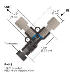
For fine control of fluid flow rates, Micro-Metering Valves can reduce outgoing flow to as low as 3.5 µL/min\*. These needle valves are perfect for use with peristaltic pump fluid-transfer applications, mass spectrometry, and fraction collection.
