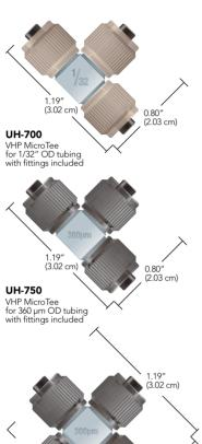
Our VHP Stainless Steel Tees and Crosses are precision machined from durable stainless steel. It is mechanically designed for bringing together three or four pieces of tubing. Our VHP Tees & Crosses have an extremely high pressure rating of 30,000 psi (2070 bar).
