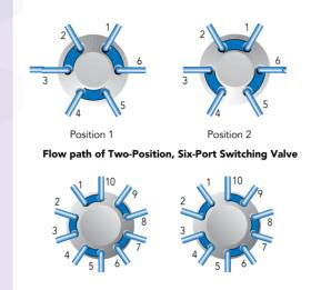
Flow path of Two-Position, Ten-Port Switching Valve
