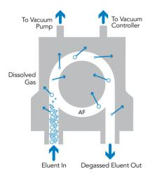
Dissolved gases are actively removed from a flowing liquid stream by vacuum via the IDEX Health & Science AF® membrane.
