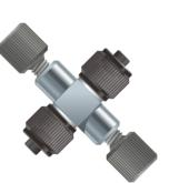
UH-906 VHP MicroTight Adapting Cross 10-32 Coned for 1/16" OD tubing and 5/16-24 Coned for 360 µm OD tubing
