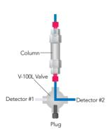
Your detector switching application may require the flexibility of routing the column effluent to both detectors simultaneously while retaining the ability to isolate each detector. Use our 3-Way Flow Switching Valve ("T"), plugging off the fourth port with the included plug.
