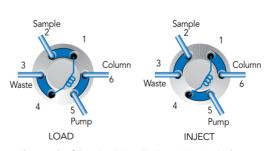
Flow path of Two-Position, Six-Port Injection Valve
