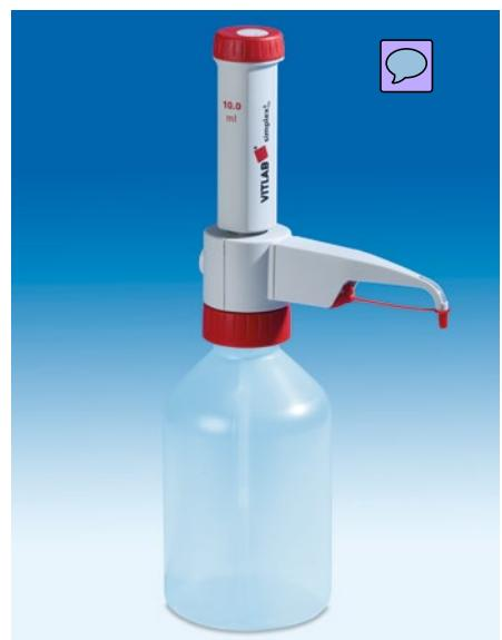
\* Nominal volume 1 - 10 ml: with adapters GL 25, GL 28, GL 32, GL 38, S 40 and telescopic intake tube (length 125 - 240 mm).
