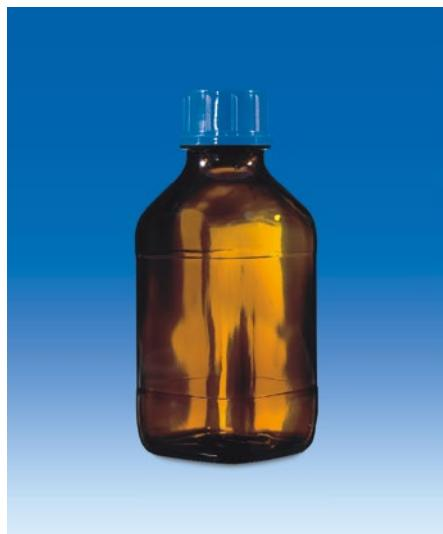
Threaded brown glass (soda lime glass) bottles with an ethylene acrylate coating for increased safety, and a screw cap. The plastic coating significantly reduces hazardous glass splintering during breakage. The maximum working temperature for coated bottles is 80 °C. To preserve the coating, do not clean at temperatures exceeding 60 °C.
