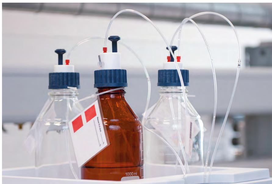
In this respect, 1000 ml solvent bottles with and without SafetyCaps were used and the emissions over a period of 28 days compared.
