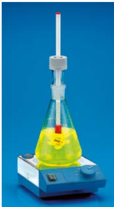
Compression-type bung made of silicone
