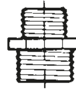
Nipple, reduced, with outer thread.
